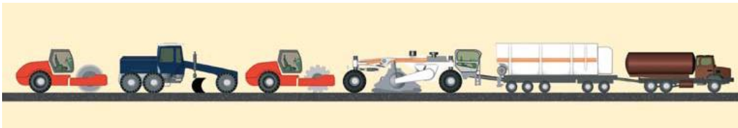
CIPR Cement and foam bitumen bonding
